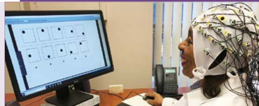
IOG staffer Odessa Jackson demonstrates the EEG cap worn by participants in Dr. Kavcic's study. The non-invasive cap measures brain waves as volunteers complete timed puzzles and other tests of cognitive abilities.
